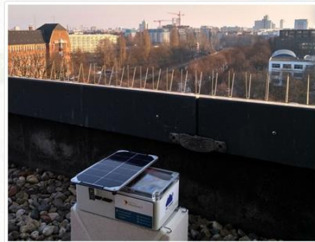
Solar powered DIY LoRaWAN weatherstation for measuring temperature and humidity.
